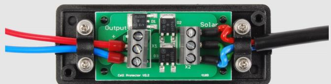
With this hookup, the cells are protected with 2 bypass diodes against the hot spot effect and the additional blocking diode protects against reverse current back into the module. By damage to a module or cable by several modules in parallel operation an influence can be prevented on the other modules with the use of the blocking diode.
