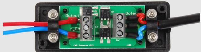
With this hookup, the cells are protected with 2 bypass diodes against the hot spot effect.
